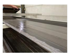
The laser head is installed above the belt on a manually controlled carriage rail and the beam is focused on an area approximately 70 mm wide. As the belt travels beneath the laser, baking residues are removed and collected by the extraction system. Once the strip has been cleaned along the full length of the belt, the laser head is moved across to the next section.
