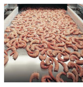
As with all food processes, hygiene is critical and the use of stainless steel belts with their ease of cleaning enables significant reductions in bacteria, yeast and mould counts compared with other belt types.
