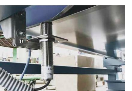
Detailed view tensioning and belt position detection system.
