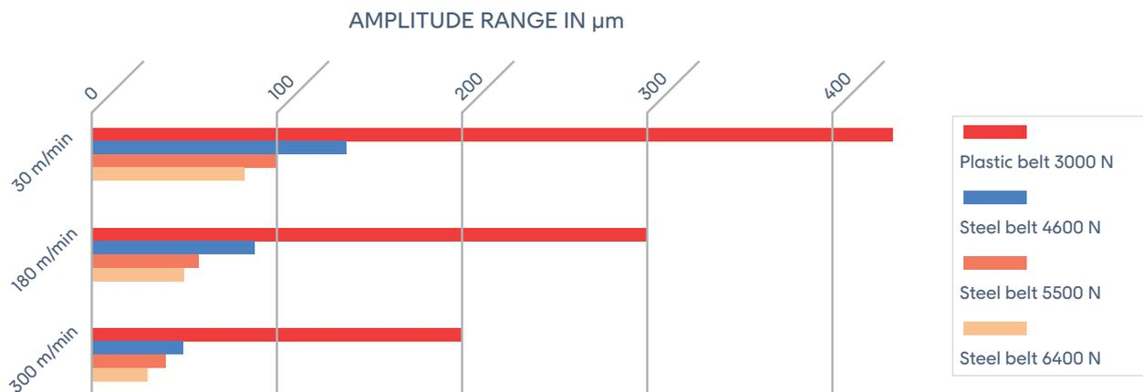
The amplitude range is the peak-to-valley value of vibrations over the measured time.  $A_{\text{range}} = [A_{\text{max}} - A_{\text{min}}]$
