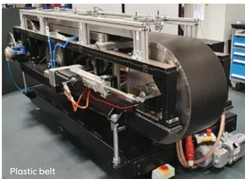
Steel belts are between 3 and 6x more stable than plastic, enabling high speed, high precision printing.
