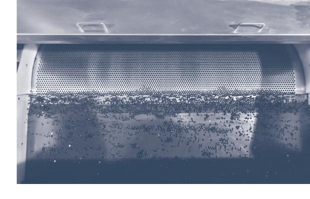
Our granulation solution is based on Rotoform technology, a system first developed in the early 1980s for the solidification of sulphur and other by-products of oil and gas refining. Since then, the IPCO Rotoform has become the standard solution for the solidification of chemicals, with more than 2 000 systems installed to date.
