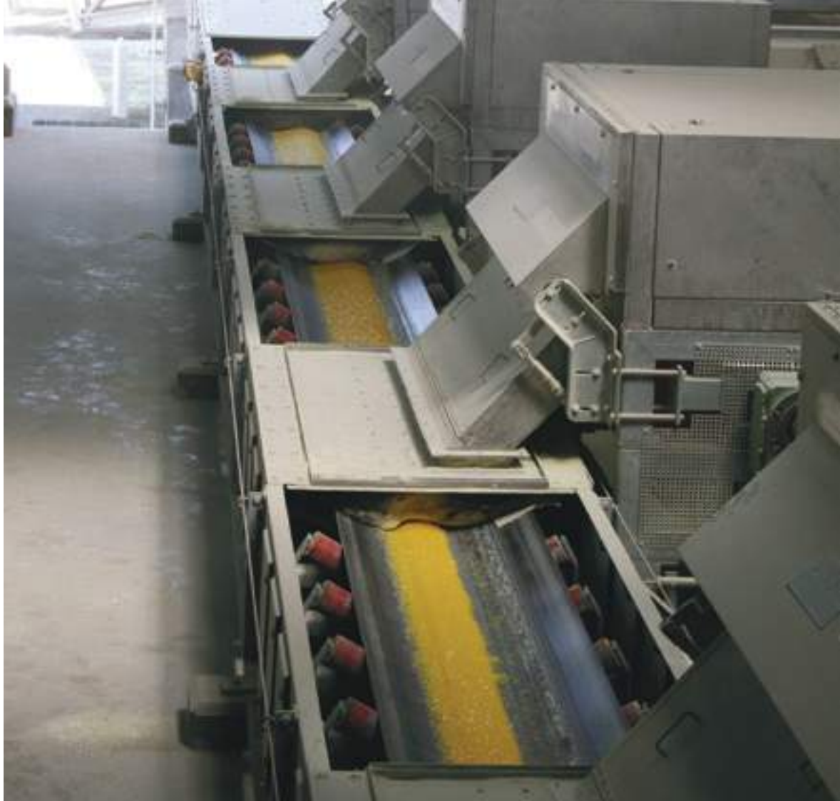
Discharge of sulphur pastilles from steel belt cooler.
