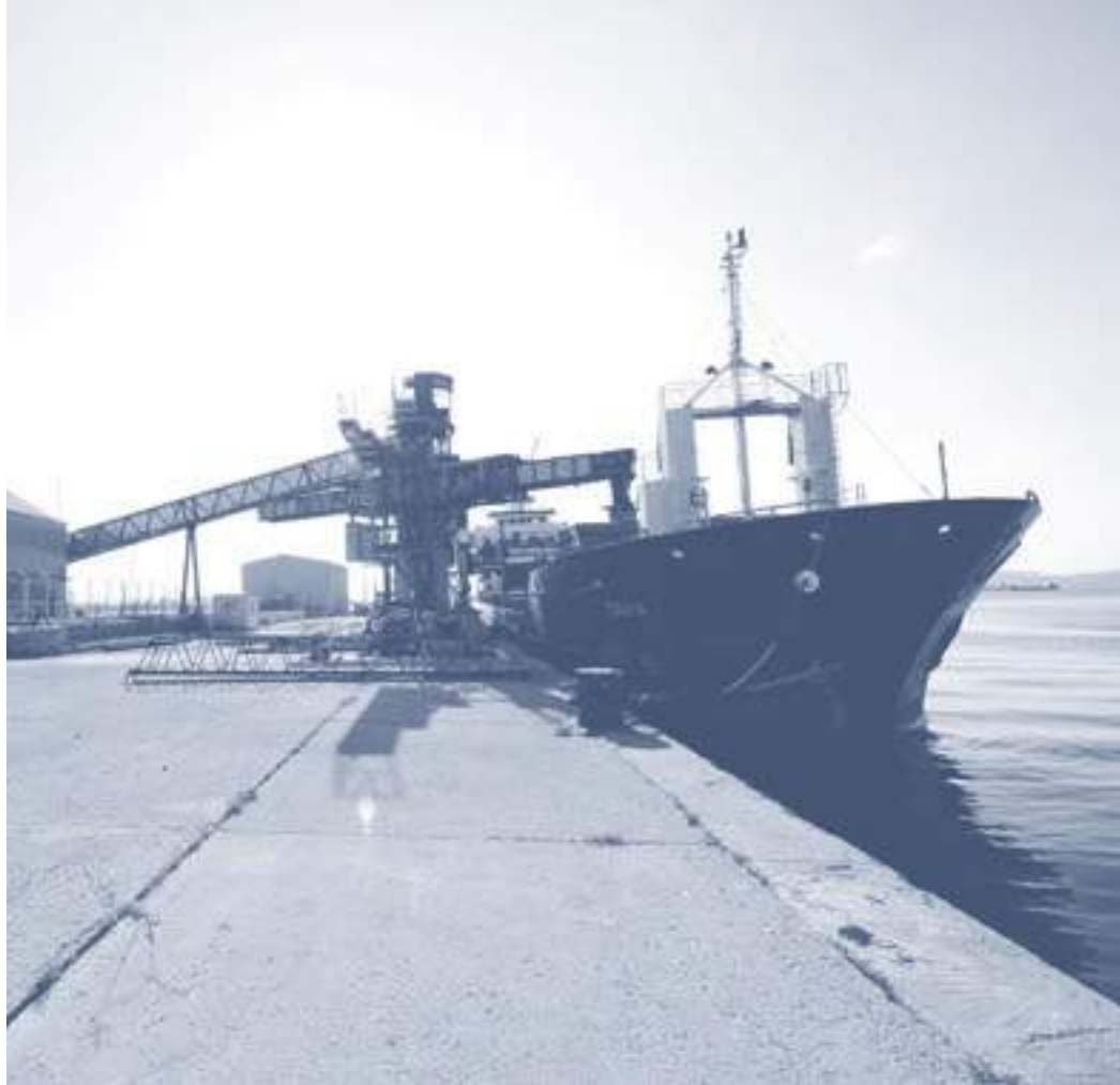
Bulk ship loading directly from an IPCO sulphur forming and storage facility.
