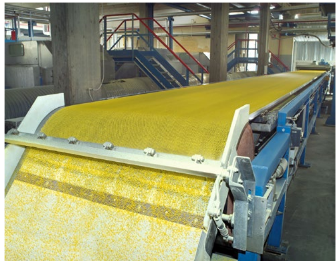
Fig. 8: A steel belt cooler producing sulphur pastilles.
