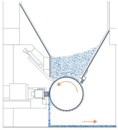
For uniform scattering of sand, silicium carbide, corundum and more.
