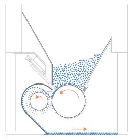
For uniform scattering of flakes, chips, granules and more.
