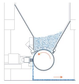
For uniform scattering of powder, mica, glitter particles, chips, flakes, sand, active carbon, glass beads and more.
