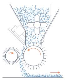
For uniform scattering of fibrous materials used in the manufacture of products for the automotive, textile, recycling and construction industries.
