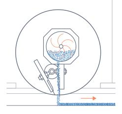
For design scatter coating applications using powder, mica, glitter particles, chips, flakes, glass, semolina, sesame and more.
