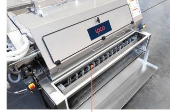
Spraying bar with nozzles.
