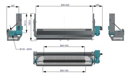
Drive power is nominal 0,37 kW, three phase 380 to 500 V/16A, 50 or 60 Hz. The actual rotational velocity can be altered by the frequency converter, which is attached to the drive. Min frequency is 13 Hz.
