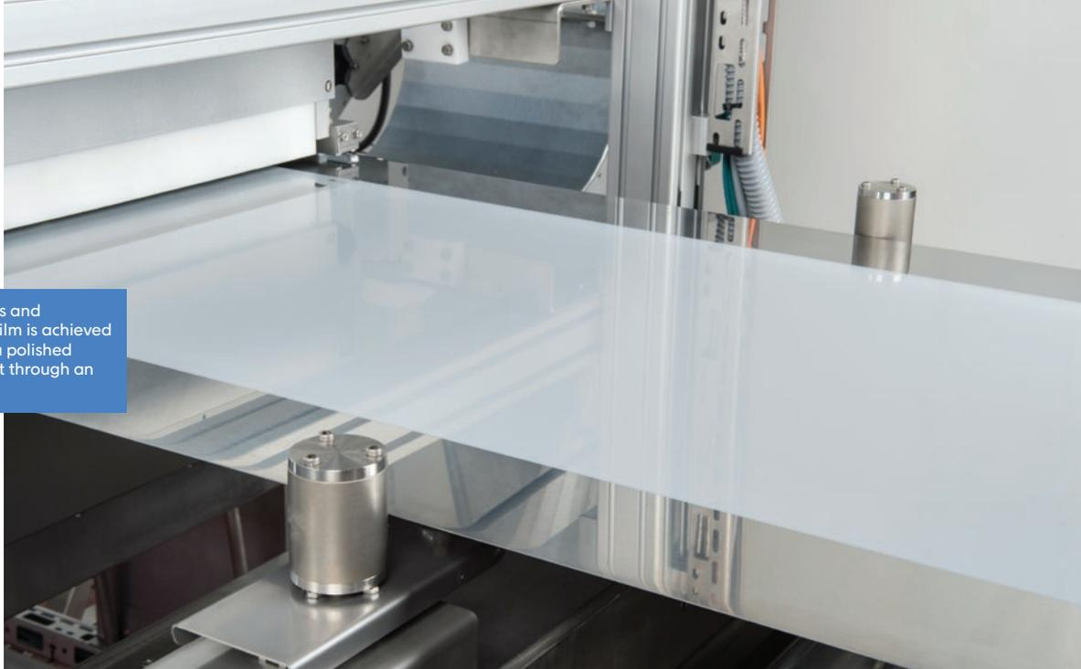
The fine tolerances of flatness and thickness required in optical film is achieved by casting liquid product on a polished IPCO steel belt then passing it through an IPCO Venturi dryer.
