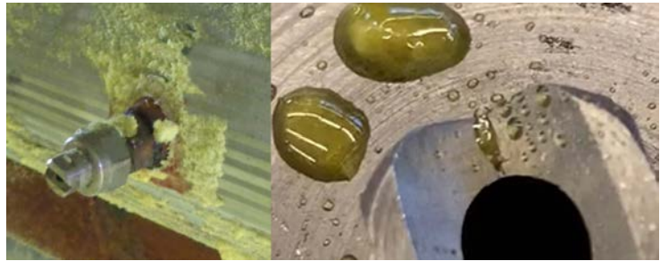
Figure 4. Unheated nozzles (left): sulfur can solidify. Heated nozzle (right): no solidification.
