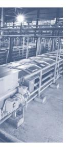
As the pastilles are taken off the end of the Rotoform line, they are conveyed outside the solidification building to the covered stockpile area.
