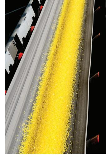
The qualities of low friability, good impact abrasion resistance, good flow characteristics, high bulk density and high angle of repose are all important, given that the solidified sulphur can be moved several times between production at the refinery and subsequent re-use (i.e. the various stages of handling, storage, shipping etc.).
