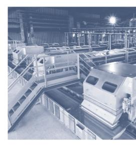
The sulphur droplets are then discharged as solid, hemispherical pastilles at the end of the cooling system. To eliminate the possibility of damage to the pastilles during discharge, a thin film of silicon-based release agent is applied to the steel belt.
