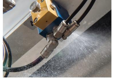
Release agent spraying system ensures easy release of pastilles from the belt
