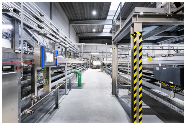
Figure 1. IPCO high-capacity Rotoform HS sulfur granulation units.
