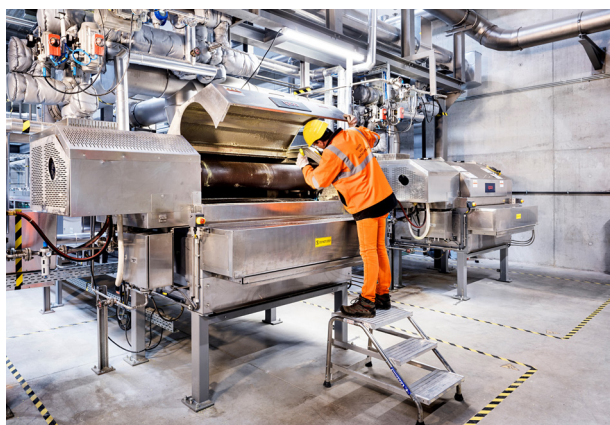
Figure 2. IPCO Rotoform feed station.
