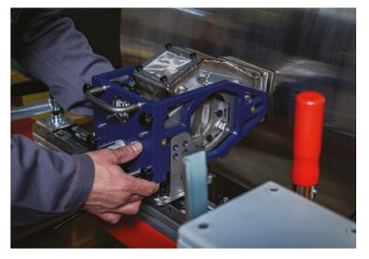
Our new Shotpeener Pro tool is used to repair deformities that can appear in a press belt over time, and can be employed without stopping production or dismantling the belt.
