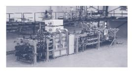
This press delivers the best of both worlds. PTFE-coated belts are used through the system, but significantly greater pressure can be applied via steel belt modules in the consolidation zone.
