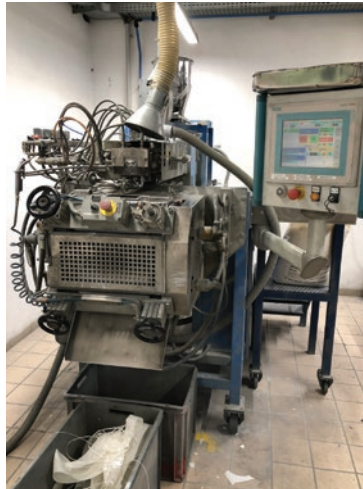
This OMC 25/29 with calender cooling system underwent a complete mechanical and electrical refurbishment
