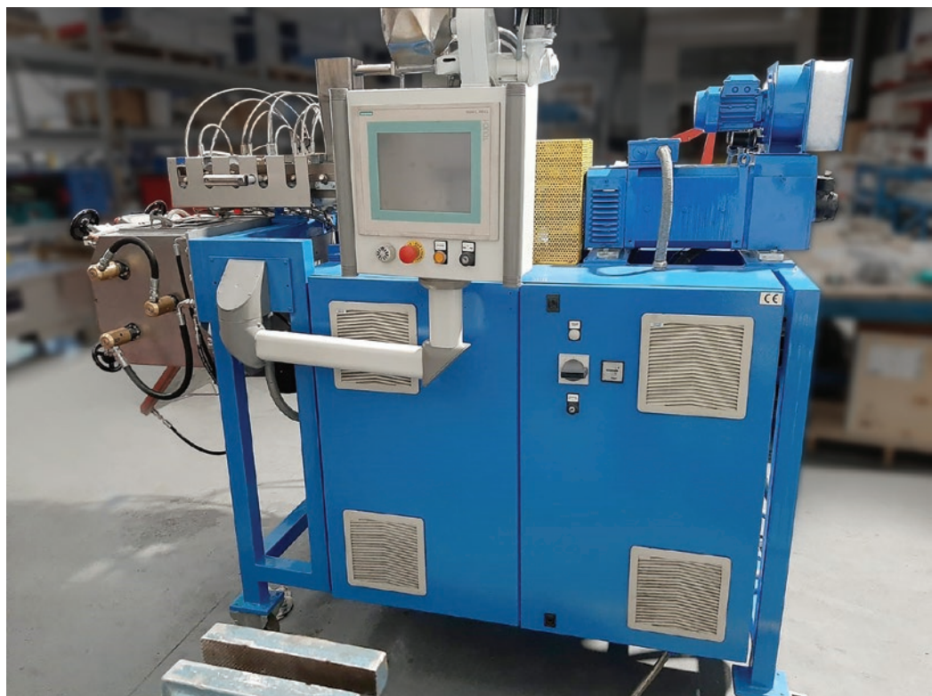
IPCO's engineers carried out a complete mechanical and electrical refurbishment of this old OMC 25/29
