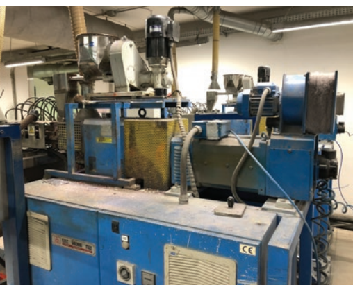
IPCO's engineers carried out a complete mechanical and electrical refurbishment of this old OMC 25/29
